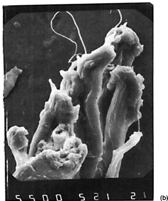
Figure 6 SEM micrographs of tensile fracture surface of polyethylene fibers irradiated in air (note that there are two fiber ends).
